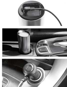
1. Insert the on-board charger into the bottom power supply interface of the PureAir.
