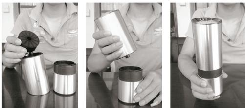
a.) Firmly hold the two metal parts of the unit. Gently turn it in opposite directions. The unit will separate in to two units. Turn over the top part of the unit and place on a table. The filter is in that assembly. Remove the old filter and replace with a new one.
